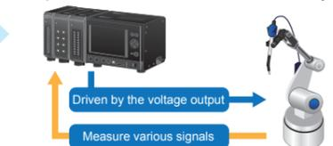
\* Signals that are being captured may not be output at the same time. The output current is max 10mA for each channel. Total output current of the unit is 40mA. If the target object needs to be driven by external power, than a power amplifier may be needed.
