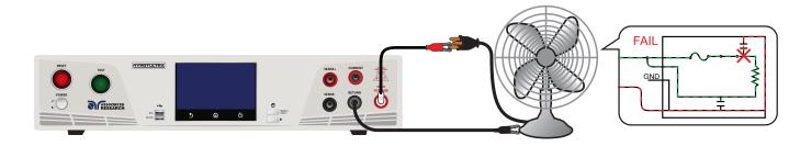
Dielectric breakdown is defined as the failure of insulation to prevent the flow of current. The best indication of dielectric breakdown is a leakage current measurement significantly higher than the nominal current measurement. The maximum leakage current is dependent upon the test voltage; therefore, the leakage current will vary depending upon the product being tested.
