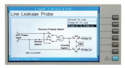
Figure 2: Leakage Current Configuration Diagram from OMNIA II
