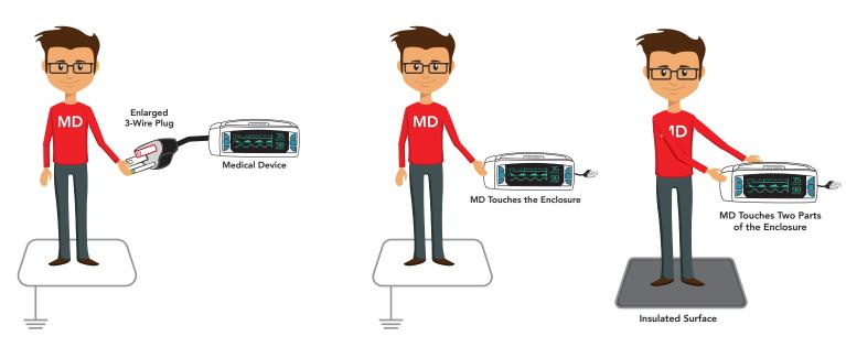
Figure 3 Earth Leakage Test
